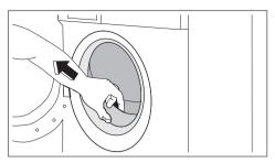
6. Fill the smaller upper hole and the two large ones with the corresponding plastic plug caps supplied in the bag containing the instruction booklet.
